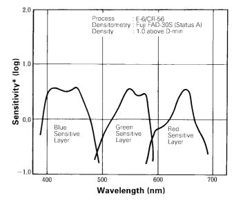
\* Sensitivity equals the reciprocal of the exposure (ergs/cm<sup>2</sup>) required to produce a specified density.
